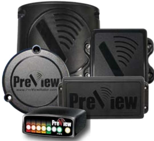
**Prevent Collisions:** PreView Radar is a pulsed radar object detection sensor designed to detect moving and stationary objects in operator blind spots. Distance to the nearest object is relayed to the in-cab display. This display provides both an audible tone that increases in speed as an object becomes closer and visual LED lights.
